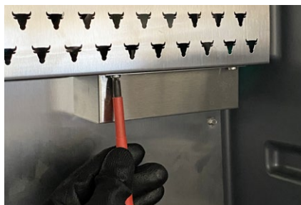
9. Screw the cover back into place.
