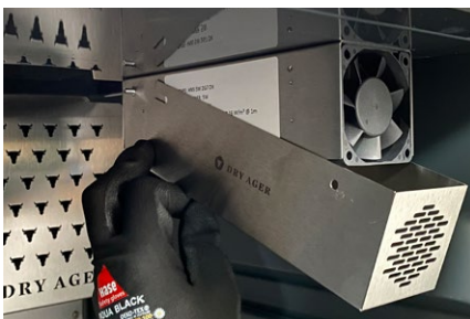
8. Slide the cover back onto the rear holding.
