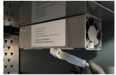
7. Pull out the old UVC bulb carefully then carefully insert the replacement UVC bulb. Do not remove the outer plastic cover of the replacement UVC bulb.
